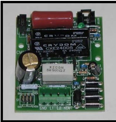
Fig 3. Showing the circuit board found on the clock movement where the movement wires connect. Note: Lead from ground on terminal plug must by connected to good ground on building electrical system.
